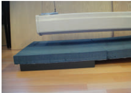
▲ Fig. 3 Absorber placed between the measurement array and the antenna under test.
