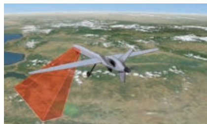
▲ Fig. 9 UAVs represent one of the most demanding and growing applications for a multitude of low SWaP-C electronically scanned antennas.
